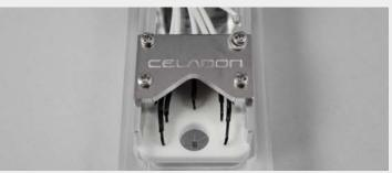
MiniTile<sup>™</sup> and WedgeTile<sup>™</sup> are economical modeling and characterization probe cards that perform with low capacitance, ultra low leakage, and fast settling times with AttoFast<sup>™</sup>.
