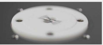
T40 ceramic probe cards have excellent performance with low noise and fast settling times, even in high temperatures.
