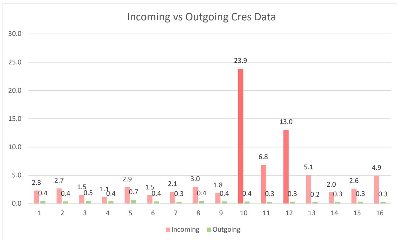
After the card is received at Celadon the card goes through an alcohol and hot water bath, followed by clean air dry, then baked for 2-4 hrs. This bath/bake process of the PM cleans to manage leakage. The Cres management is accomplished by touching down the probe card on a Tungsten Carbide [WC] substrate or Celadon Tungsten Carbide Cleaning Wafer. For best results with Tungsten Carbide cleaning substrate **the overdrive used on the substrate should match that of your test environment.**
