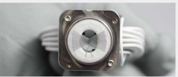
TV19 VersaTile™ probe cards are designed with Celadon's patented ceramic technology for superior electrical performance, yet is highly modular due to it's 28mm x 28mm chassis.
