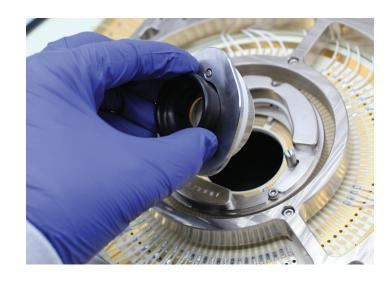
The VC43<sup>™</sup> can be used for production parametric test, modeling, characterization, and wafer level reliability testing. Cards can be configured up to 104 probes in either single or dual layer with near vertical probes to minimize scrub lengths on pads allowing the VC43<sup>™</sup> to probe pads as small as 27µm.
