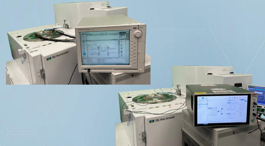
B_Tool and S_Tool are connected to Celadon Probe system (VC20)
